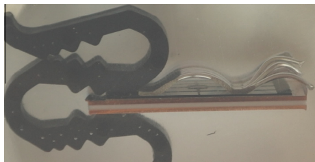
Fig. 3. IGBT chip cast into epoxy and subjected to polishing until a side view of the wire interface is reached.
